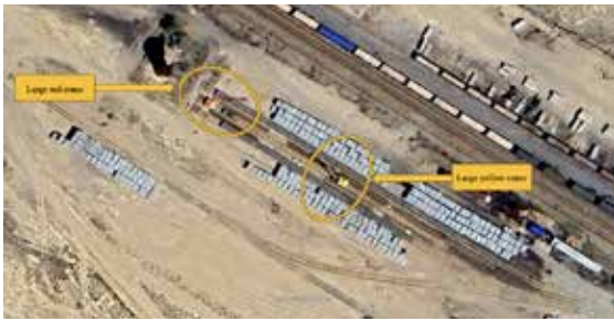
Figure 3c: Close up of the Orta Deresin supply depot site showing the concrete ties and construction machinery in more detail. Notice the large yellow and red cranes near the concrete tie stacks. Coordinates 46°49'29.94"N 75°13'28.10"E Source: Google Earth.
