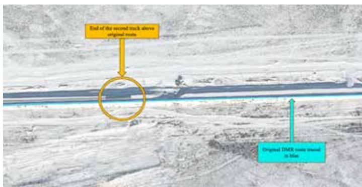
Figure 6: The end of the laid new track on January 17, 2024. Despite the snow, the truck paths to the north of the railway, the numerous access points, and the flatly graded rail bed are still visible. Copyright Maxar 2024. Coordinates 46.81846, 77.67652
