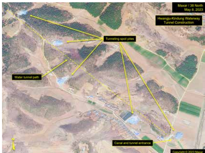
Figure 2: Tunneling spoil piles visible along water tunnel path on imagery from May 8, 2023 Source: Copyright © 2023 by Maxar
