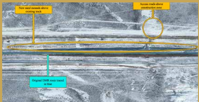
Figure 5a: Track construction in progress on 3 January 2024. Note the line of sand heaps to the north of the existing track, robust roadway above them, and regular access routes to the leveled ground above the track. Coordinates: 46.83483, 77.84664 Source: Copyright Maxar 2024.
