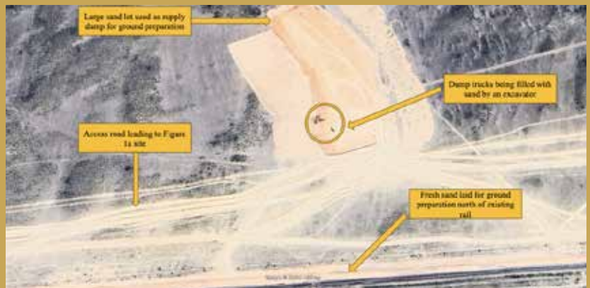
Figure 4b: Imagery of a forward sandlot along the construction site, dump truck and excavators, and the access road. Coordinates 46°55'27.46"N 74°17'15.81"E Source: Google Earth, May 12, 2023,
