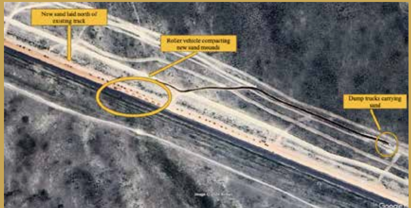
Figure 4a: Imagery of the new sand base being laid and compacted north of the existing rail. Coordinates 46°55'27.46"N 74°17'15.81"E Source: Google Earth, May 12, 2023
